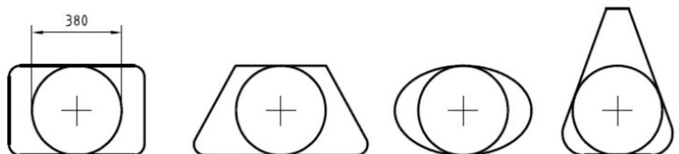
**3.08 Figure 1 - Measurements of Minimum Clear Opening Hatches & Companionways**
