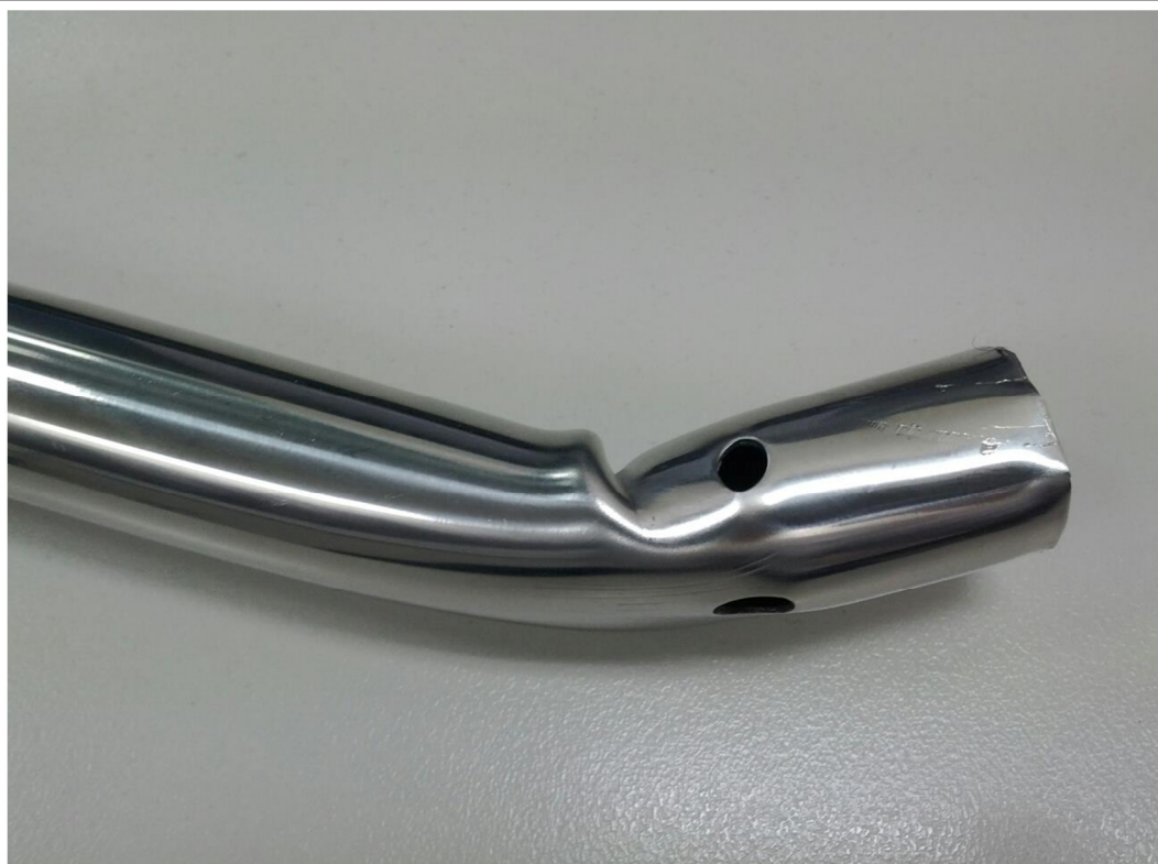
Stainless Steel. The stainless steel has deformed significantly.
