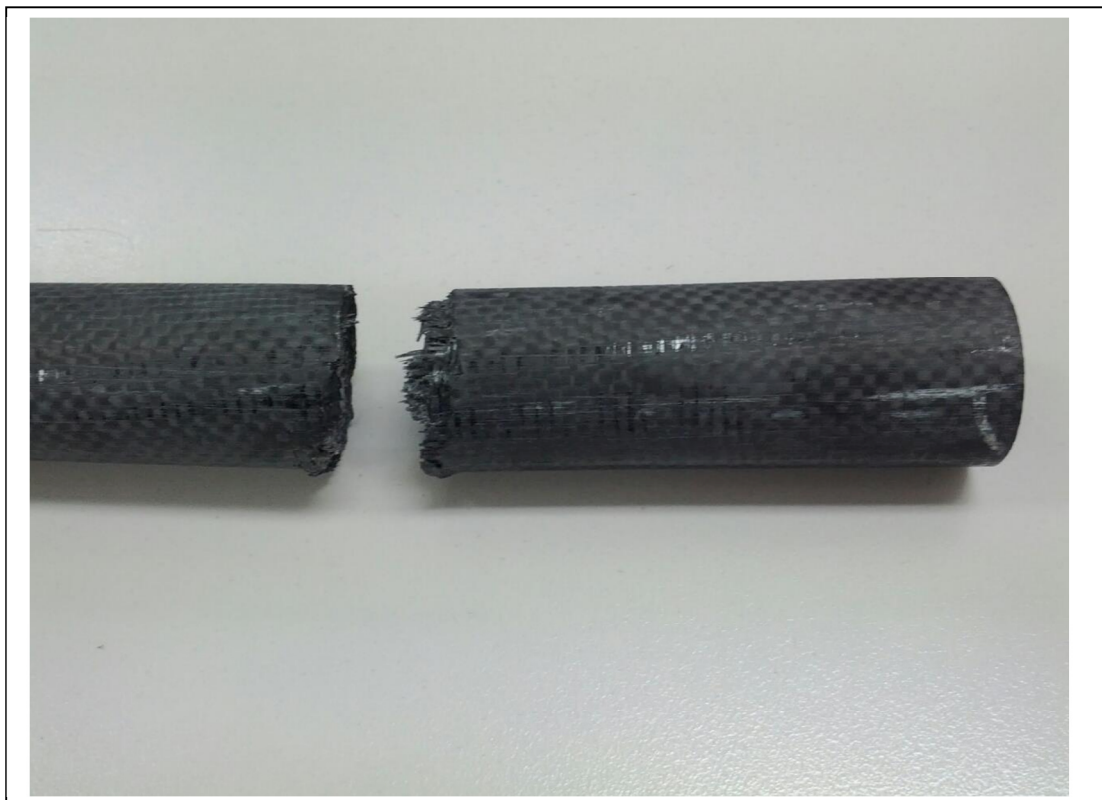
Carbon fibre/E-glass. Rough tears can be seen where the break has occurred. This is evident on the full circumference of the stanchion.
