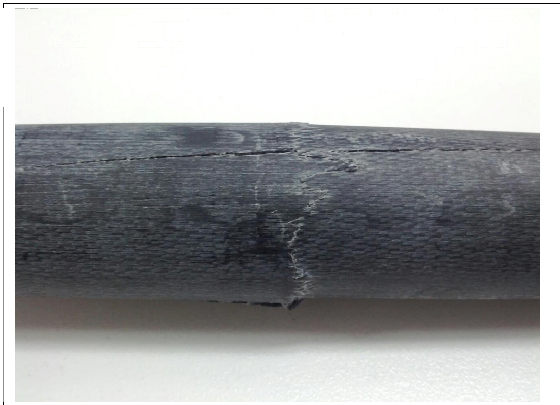
E-glass. Closer viewing shows velar vertical splits in the E-glass.
