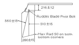
3.7 The dimensions of the **rudder** blade shall conform with the diagram. The **rudder** blade shall be not more than 14mm thick and the thickness shall not vary by more than 1mm to within 25mm of its edges with the exception of hollows or cavities of not more than 2mm in dimension and holes for fixing.
