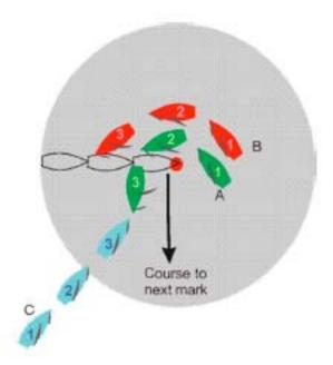
A (Green) on starboard tack leeward is overlapped to B (Red) at the zone on a windward mark to be left on port. C (Blue) is approaching the mark on port tack. A is rounding the mark as she would do in the absence of the boats B and C. By changing her course at the mark to a downwind course A comes to a collision course with C, without giving C room to keep clear.
